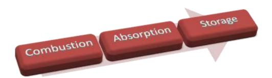
The synthesis of HCl is performed by combustion of hydrogen and chlorine gas. Both the reaction and the absorption of heat in water are highly exothermic. The HCl gas formed is absorbed in demineralized water to produce HCl acid which is then stored in rubberlined steel tanks.
