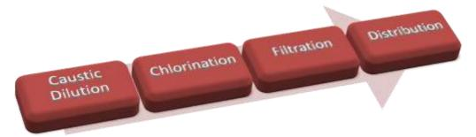
Caustic soda is diluted with demineralized water to attain 10-11% concentration. Gaseous chlorine is then added in the chlorination process producing sodium hypochlorite. The solution undergoes a series of filtration process to remove any contaminants. Finally, it is stored in the storage tanks ready for distribution.
